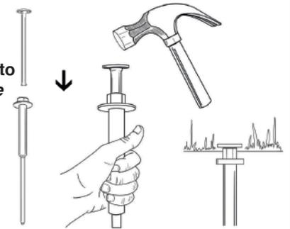
5. Place the Pole Adapter into the Ground Sleeve. Next, place the flag onto the Pole Adapter. When not in use, place the Ground Cap into the Ground Sleeve. Note: If using the 24" Pole Adapter Extension, insert into Ground Sleeve and then place Pole Adapter and flag atop of Extension.
