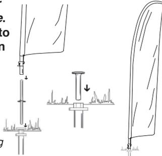
6. To Remove: Thread Extractor Tee into Ground Sleeve, slide Driving Rod through Extractor Tee and pull Ground Sleeve from the ground.
