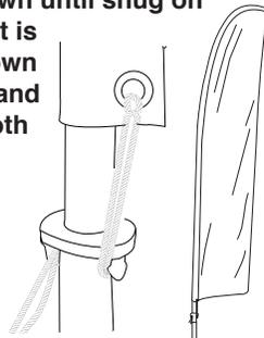
4. Next, install the ground sleeve system by placing the Driving Rod into the Ground Sleeve and drive sleeve into ground until top of nut is flush with the earth.
