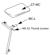
Side counter supports should be attached to side of main frame so that top of support is 39" from ground. Then attach counter top to support with thumb screws.
